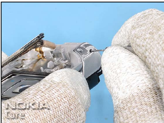
23. Compress the spring of the HINGE with the SS-6...
