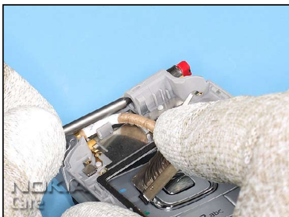
25. The HINGE can be pushed out with a Torx bit...
