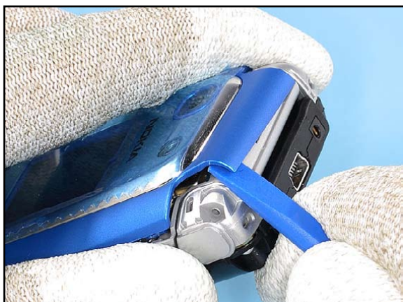
7. Gently detach the A-COVER ASSY, beginning on the top side with the SS-93.
