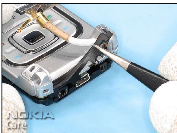
29. For the replacement of the COAX CABLE the upper and the lower block must be disassembled. Also the HINGE STOP must be removed. The disassembly procedure is now completed.
