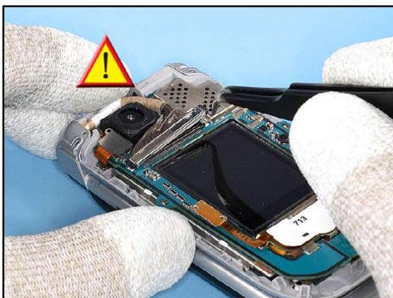
12. Lever up the COAX ASSEMBLY with the angled tweezers. It is very important not to bend these connector, otherwise it becomes unusable.
