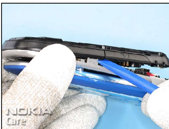
12. Unlock the clips of the D-COVER...
