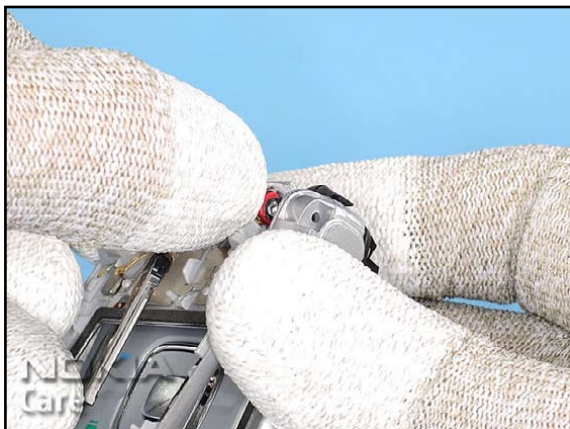
24. ...and lift the now released side of the C-COVER. Hold the HINGE into position while moving the C-COVER.
