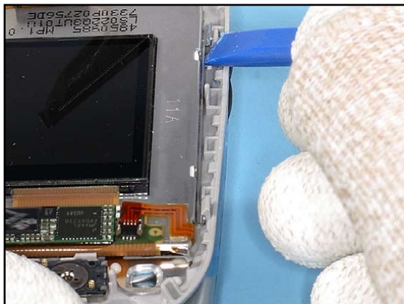
20. Unlock the plastic clips of the LCD MODULE.
