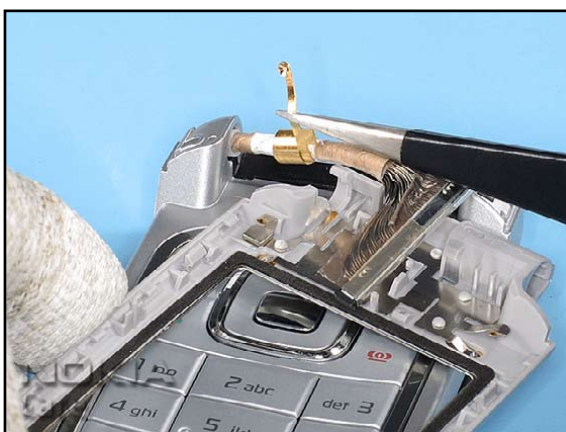
28. Carefully pull out the coax grounding clip.
