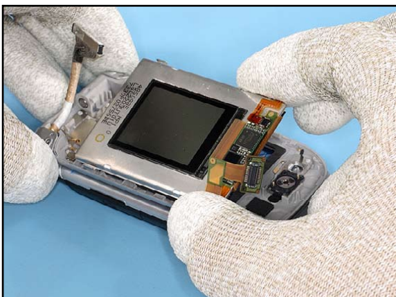
21. Now flip out the LCD MODULE.
