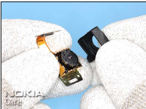
19. The CAMERA GASKET can be removed.
