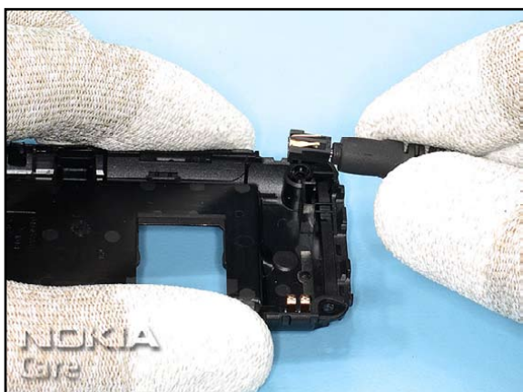
21. Lift out the connector with the DC PLUG.
