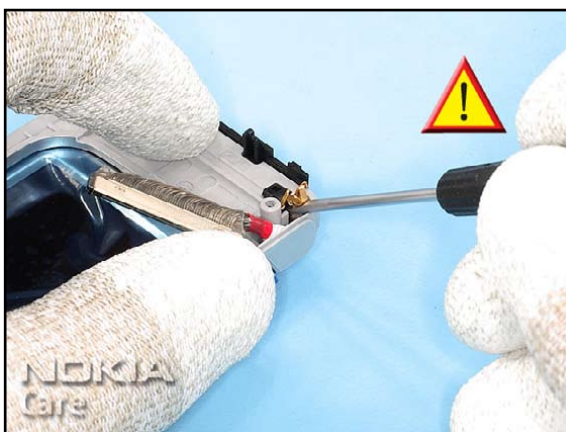
22. Ease out the HINGE GROUNDING CLIP carefully with a straight bladed screwdriver.. Do not scratch the coax cable underneath.
