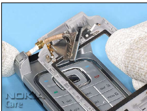
27. Note that the parts are still connected with the coax cable.
