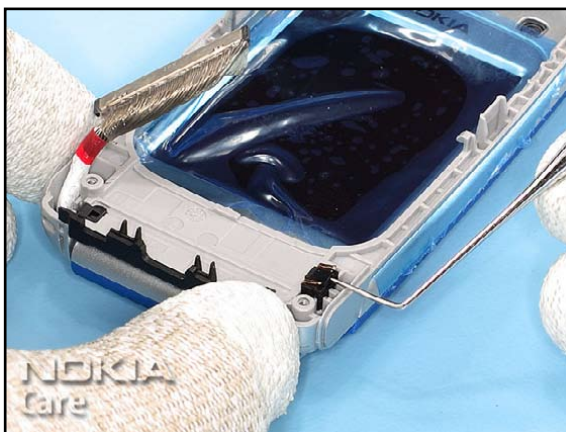
24. Ease out the MICROPHONE with the dental pick.
