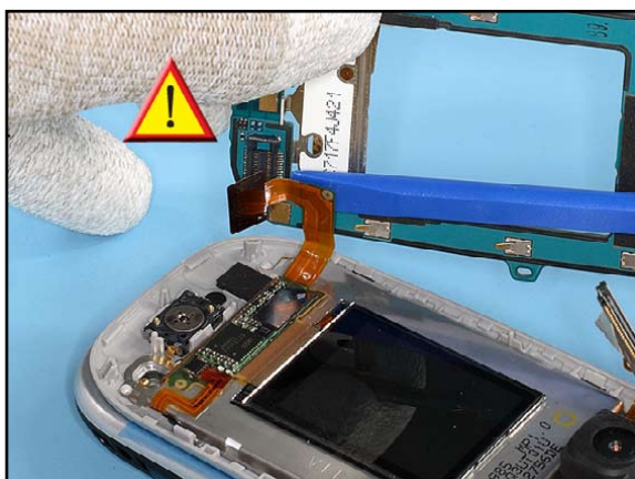
15. Flip over the TOP BOARD MECH ASSY now. Disconnect the flex connector with the SS-93.
