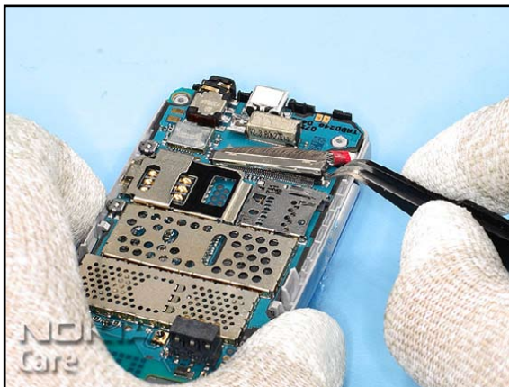
16. Carefully open the connector as shown.
