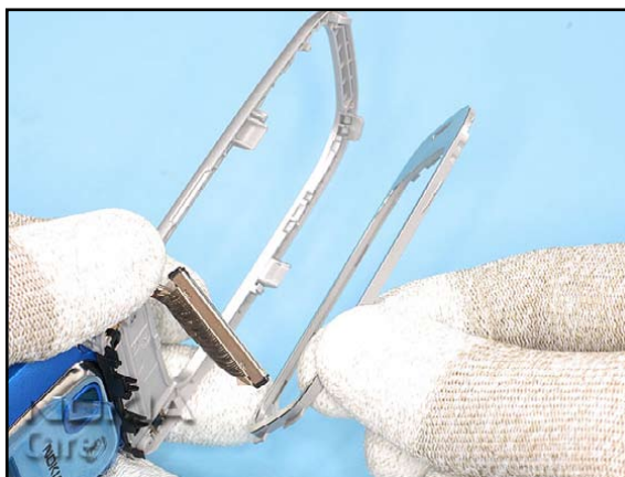
20. Also remove the KEYMAT FRAME ASSY.
