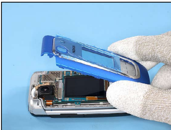
10. Now lift up the A-COVER ASSY, beginning from the hinge side in order to release the last 2 clips.
