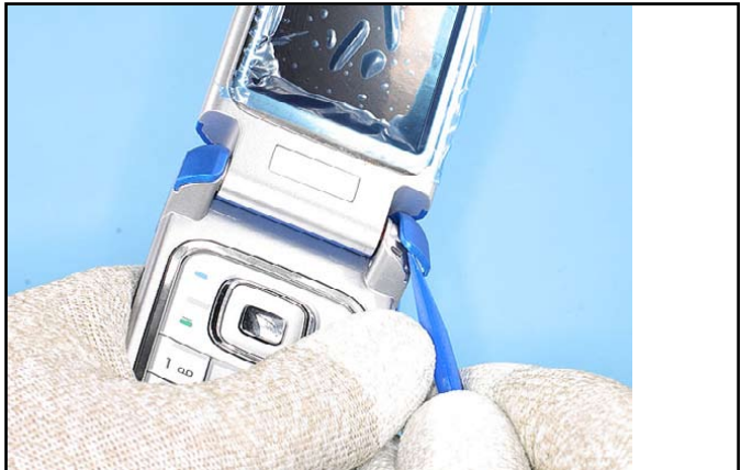
4. Unlock the clips of the SHOULDER CAP...
